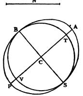
For we have stated before this, that the line N being the radius of a spherical wave of light in air, while in the crystal it spread through the spheroid ABPS, the ratio of N to CS will be 156,962 to 93,410. But it has also been stated that the proportion of the regular refraction was 5 to 3; that is to say, that N being the radius of a spherical wave of light in air, its extension in the crystal would, in the same space of time,
