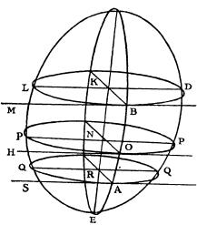
which, in cutting the spheroid make the ellipses LBD, POP, QAQ; which will all be similar and similarly disposed, and will have their centres K, N, R, in one and the same diameter of the spheroid, which will also be the diameter of the ellipse made by the section of the plane that passes through the centre of the spheroid, and which cuts the planes of the three said Ellipses at right
