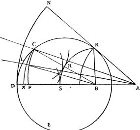
case this oval becomes a perfect circle, namely when the ratio of AD to DB is the same as the ratio of the refractions, here as 3 to 2, as I observed a long time ago. The 4th oval, serving only for impossible reflexions, there is no need to set it forth.
