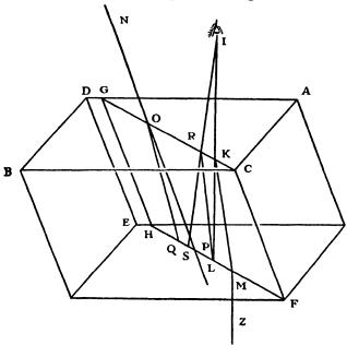
8. But in order to explain these phenomena more particularly, let there be, in the first place, a piece ABFE of the same Crystal, and let the obtuse angle ACB, one of the three which constitute the equilateral solid angle C, be divided into two equal parts by the straight line CG, and let it be conceived that the Crystal is intersected by a plane which passes through this line and through the side CF, which plane will necessarily be perpendicular to
