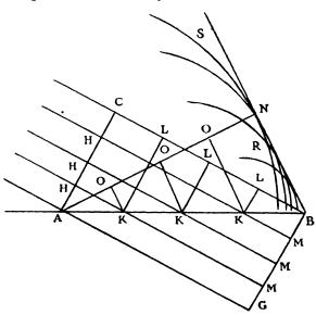
in a certain space of time advance as far as the plane AB at B, following the straight line CB, which may be supposed to come from the luminous centre, and which in consequence is perpendicular to AC. Now in this same space of time the portion A of the same wave, which has been hindered from communicating its movement beyond the plane AB, or at least partly so, ought to have continued its movement in the matter which is above this plane, and this along a distance equal to CB, making its
