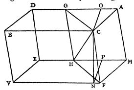
and CO perpendicular to DA. This angle OCN I found to be 105 degrees; and its supplement CNP, to be 75 degrees, as it should be.
