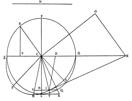
is RC to CV. But KO is equal to N, and RC to CG: then as CK is to N so will CG be to CV. But as N is to CG, so, by construction, is CV to CD. Then as CK is to CG so is CG to CD. And because DI is parallel to CM, the conjugate diameter to CG, it follows that KI touches the Ellipse at I; which remained to be shown.
