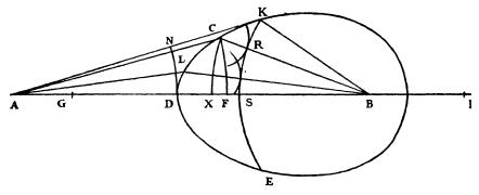
reflexion or by refraction, it is only necessary to make this surface such that the path of the light from the point A to all points of the curved line CDE, and from these to the point of concurrence (as here the path along the straight lines AC, CB, along AL, LB, and along AD, DB), shall be everywhere traversed in equal times: by which principle the finding of these curves becomes very easy.
