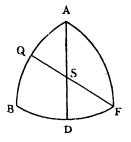
FQA has a right angle at Q, the angle A 105 degrees, and F half as much, namely 52 degrees 30 minutes; whence the hypotenuse AF is found to be 101 degrees 52 minutes. And this arc AF is the measure of the angle ACF in the figure of the crystal.
