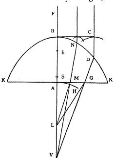
be found. And this line being then prolonged at one side or the other will meet the straight line BL, as here at V. Let there then be erected on AB the perpendicular BC, which will represent a wave of light coming from the infinitely distant point F, since we have supposed the rays to be parallel. Then all the parts of this wave BC must arrive at the same time at the point L; or rather all the parts of a wave emanating from the point L must
