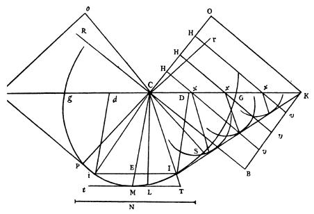
refraction of the ray RC is nothing else than the progression of the portion C of the wave CO, continued in the crystal. Now the portions H of this wave, during the time that O came to K, will have arrived at the surface CK along the straight lines Hx, and will moreover have produced in the crystal around the centres x some hemispheroidal partial waves similar to the hemispheroidal GSPg, and similarly disposed, and of which the major and
