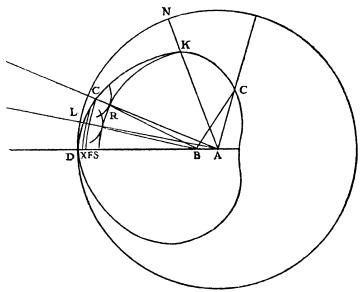
Ovals the first of which we have already set forth. The second oval is that which serves for rays that tend to a given point; in which oval, if the apex of the surface which receives the rays is D, it will happen that the other apex will be situated between B and A, or beyond A, according as the ratio of AD to DB is given of greater or lesser value. And in this latter case it is the same as that which Des Cartes calls his 3rd oval.
