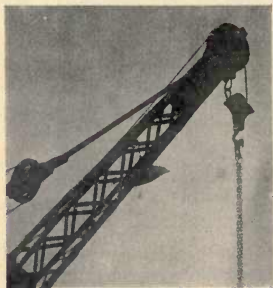
FIG. 44. Crane showing lattice (girder) shaft and solid head.
